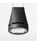
Suspended luminaire with LED, rated life of the LED L80/B10 > 50000 h, colour rendering index CRI > 82, chromaticity tolerance 2 SDCM (initial), reflector with circular light distribution pattern, reflector pure aluminium 99,99% in MIRO-Silver®, canopy sheet steel, powder-coated, luminaire head die-cast aluminium, powder-coated, black
