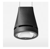
Suspended luminaire with LED, rated life of the LED L80/B10 > 50000 h, colour rendering index CRI > 90, chromaticity tolerance 2 SDCM (initial), reflector with circular light distribution pattern, reflector pure aluminium 99,99% in MIRO-Silver®, canopy sheet steel, powder-coated, luminaire head die-cast aluminium, powder-coated, black
