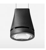
Suspended luminaire with LED, rated life of the LED L80/B10 > 50000 h, colour rendering index CRI > 90, chromaticity tolerance 2 SDCM (initial), reflector with circular light distribution pattern, reflector pure aluminium 99,99% in MIRO-Silver®, canopy sheet steel, powder-coated, luminaire head die-cast aluminium, powder-coated, black
