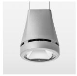
Suspended luminaire with LED, rated life of the LED L80/B10 > 50000 h, colour rendering index CRI > 80, chromaticity tolerance 2 SDCM (initial), reflector with circular light distribution pattern, reflector pure aluminium 99,99% in MIRO-Silver®, canopy sheet steel, powder-coated, luminaire head die-cast aluminium, powder-coated, silver
