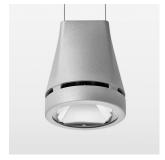
Suspended luminaire with LED, rated life of the LED L80/B10 > 50000 h, colour rendering index CRI > 90, chromaticity tolerance 2 SDCM (initial), reflector with circular light distribution pattern, reflector pure aluminium 99,99% in MIRO-Silver®, canopy sheet steel, powder-coated, luminaire head die-cast aluminium, powder-coated, silver
