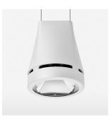
Suspended luminaire with LED, rated life of the LED L80/B10 > 50000 h, colour rendering index CRI > 80, chromaticity tolerance 2 SDCM (initial), reflector with circular light distribution pattern, reflector pure aluminium 99,99% in MIRO-Silver®, luminaire head die-cast aluminium, powder-coated, white, separate driver unit
