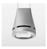
Suspended luminaire with LED, rated life of the LED L80/B10 > 50000 h, colour rendering index CRI > 82, chromaticity tolerance 2 SDCM (initial), reflector with circular light distribution pattern, reflector pure aluminium 99,99% in MIRO-Silver®, canopy sheet steel, powder-coated, luminaire head die-cast aluminium, powder-coated, silver
