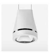
Suspended luminaire with LED, rated life of the LED L80/B10 > 50000 h, colour rendering index CRI > 70, chromaticity tolerance 2 SDCM (initial), reflector with circular light distribution pattern, reflector pure aluminium 99,99% in MIRO-Silver®, canopy sheet steel, powder-coated, luminaire head die-cast aluminium, powder-coated, white
