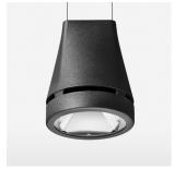
Suspended luminaire with LED, rated life of the LED L80/B10 > 50000 h, colour rendering index CRI > 80, chromaticity tolerance 2 SDCM (initial), reflector with circular light distribution pattern, reflector pure aluminium 99,99% in MIRO-Silver®, canopy sheet steel, powder-coated, luminaire head die-cast aluminium, powder-coated, black
