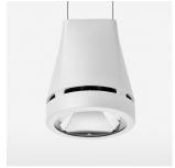
Suspended luminaire with LED, rated life of the LED L80/B10 > 50000 h, colour rendering index CRI > 80, chromaticity tolerance 2 SDCM (initial), reflector with circular light distribution pattern, reflector pure aluminium 99,99% in MIRO-Silver®, canopy sheet steel, powder-coated, luminaire head die-cast aluminium, powder-coated, white
