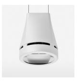
Suspended luminaire with LED, rated life of the LED L80/B10 > 50000 h, colour rendering index CRI > 80, chromaticity tolerance 2 SDCM (initial), reflector with oval light distribution pattern, reflector pure aluminium 99,99% in MIRO-Silver®, luminaire head die-cast aluminium, powder-coated, white, separate driver unit
