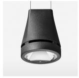
Suspended luminaire with LED, rated life of the LED L80/B10 > 50000 h, colour rendering index CRI > 70, chromaticity tolerance 2 SDCM (initial), reflector with circular light distribution pattern, reflector pure aluminium 99,99% in MIRO-Silver®, luminaire head die-cast aluminium, powder-coated, black
