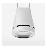
Suspended luminaire with LED, rated life of the LED L80/B10 > 50000 h, colour rendering index CRI > 80, chromaticity tolerance 2 SDCM (initial), reflector with oval light distribution pattern, reflector pure aluminium 99,99% in MIRO-Silver®, canopy sheet steel, powder-coated, luminaire head die-cast aluminium, powder-coated, white
