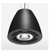
Suspended luminaire with LED, rated life of the LED L80/B10 > 50000 h, colour rendering index CRI > 82, chromaticity tolerance 2 SDCM (initial), reflector with circular light distribution pattern, reflector pure aluminium 99,99% in MIRO-Silver®, swivel angle +/-25°, luminaire housing sheet steel, powder-coated, black
