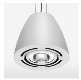
Suspended luminaire with LED, rated life of the LED L80/B10 > 50000 h, colour rendering index CRI > 90, chromaticity tolerance 2 SDCM (initial), reflector with oval light distribution pattern, reflector pure aluminium 99,99% in MIRO-Silver®, swivel angle +/-25°, luminaire housing sheet steel, powdercoated, white
