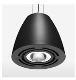
Suspended luminaire with LED, rated life of the LED L80/B10 > 50000 h, colour rendering index CRI > 90, chromaticity tolerance 2 SDCM (initial), reflector with oval light distribution pattern, reflector pure aluminium 99,99% in MIRO-Silver®, swivel angle +/-25°, luminaire housing sheet steel, powder-coated, black
