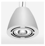
Suspended luminaire with LED, rated life of the LED L80/B10 > 50000 h, colour rendering index CRI > 80, chromaticity tolerance 2 SDCM (initial), reflector with oval light distribution pattern, reflector pure aluminium 99,99% in MIRO-Silver®, swivel angle +/-25°, luminaire housing sheet steel, powder-coated, white
