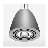
Suspended luminaire with LED, rated life of the LED L80/B10 > 50000 h, colour rendering index CRI > 80, chromaticity tolerance 2 SDCM (initial), reflector with oval light distribution pattern, reflector pure aluminium 99,99% in MIRO-Silver®, swivel angle +/-25°, luminaire housing sheet steel, powder-coated, silver
