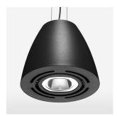
Suspended luminaire with LED, rated life of the LED L80/B10 > 50000 h, colour rendering index CRI > 80, chromaticity tolerance 2 SDCM (initial), reflector with oval light distribution pattern, reflector pure aluminium 99,99% in MIRO-Silver®, swivel angle +/-25°, luminaire housing sheet steel, powder-coated, black
