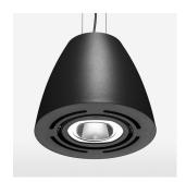
Suspended luminaire with LED, rated life of the LED L80/B10 > 50000 h, colour rendering index CRI > 82, chromaticity tolerance 2 SDCM (initial), reflector with circular light distribution pattern, reflector pure aluminium 99,99% in MIRO-Silver®, swivel angle +/-25°, luminaire housing sheet steel, powder-coated, black
