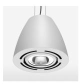
Suspended luminaire with LED, rated life of the LED L80/B10 > 50000 h, colour rendering index CRI > 82, chromaticity tolerance 2 SDCM (initial), reflector with circular light distribution pattern, reflector pure aluminium 99,99% in MIRO-Silver®, swivel angle +/-25°, luminaire housing sheet steel, powder-coated, white
