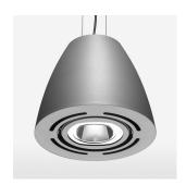
Suspended luminaire with LED, rated life of the LED L80/B10 > 50000 h, colour rendering index CRI > 80, chromaticity tolerance 3 SDCM (initial), reflector with circular light distribution pattern, reflector pure aluminium 99,99% in MIRO-Silver®, swivel angle +/-25°, luminaire housing sheet steel, powder-coated, silver
