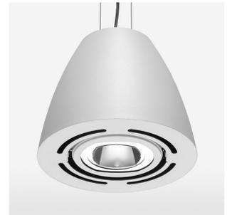
Suspended luminaire with LED, rated life of the LED L80/B10 > 50000 h, colour rendering index CRI > 90, chromaticity tolerance 2 SDCM (initial), reflector with circular light distribution pattern, reflector pure aluminium 99,99% in MIRO-Silver®, swivel angle +/-25°, luminaire housing sheet steel, powder-coated, white
