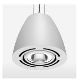
Suspended luminaire with LED, rated life of the LED L80/B10 > 50000 h, colour rendering index CRI > 80, chromaticity tolerance 3 SDCM (initial), reflector with circular light distribution pattern, reflector pure aluminium 99,99% in MIRO-Silver®, swivel angle +/-25°, luminaire housing sheet steel, powder-coated, white
