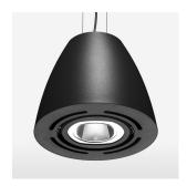
Suspended luminaire with LED, rated life of the LED L80/B10 > 50000 h, colour rendering index CRI > 90, chromaticity tolerance 2 SDCM (initial), reflector with circular light distribution pattern, reflector pure aluminium 99,99% in MIRO-Silver®, swivel angle +/-25°, luminaire housing sheet steel, powder-coated, black
