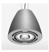
Suspended luminaire with LED, rated life of the LED L80/B10 > 50000 h, colour rendering index CRI > 90, chromaticity tolerance 2 SDCM (initial), reflector with circular light distribution pattern, reflector pure aluminium 99,99% in MIRO-Silver®, swivel angle +/-25°, luminaire housing sheet steel, powder-coated, silver
