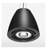
Suspended luminaire with LED, rated life of the LED L80/B10 > 50000 h, colour rendering index CRI > 90, chromaticity tolerance 2 SDCM (initial), reflector with circular light distribution pattern, reflector pure aluminium 99,99% in MIRO-Silver®, swivel angle +/-25°, luminaire housing sheet steel, powder-coated, black
