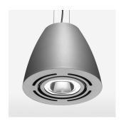
Suspended luminaire with LED, rated life of the LED L80/B10 > 50000 h, colour rendering index CRI > 80, chromaticity tolerance 2 SDCM (initial), reflector with circular light distribution pattern, reflector pure aluminium 99,99% in MIRO-Silver®, swivel angle +/-25°, luminaire housing sheet steel, powder-coated, silver
