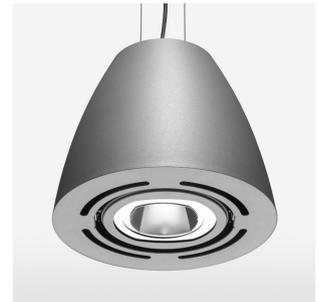
Suspended luminaire with LED, rated life of the LED L80/B10 > 50000 h, colour rendering index CRI > 80, chromaticity tolerance 2 SDCM (initial), reflector with circular light distribution pattern, reflector pure aluminium 99,99% in MIRO-Silver®, swivel angle +/-25°, luminaire housing sheet steel, powder-coated, silver
