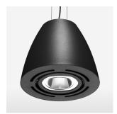
Suspended luminaire with LED, rated life of the LED L80/B10 > 50000 h, colour rendering index CRI > 80, chromaticity tolerance 3 SDCM (initial), reflector with circular light distribution pattern, reflector pure aluminium 99,99% in MIRO-Silver®, swivel angle +/-25°, luminaire housing sheet steel, powder-coated, black
