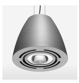
Suspended luminaire with LED, rated life of the LED L80/B10 > 50000 h, colour rendering index CRI > 80, chromaticity tolerance 2 SDCM (initial), reflector with circular light distribution pattern, reflector pure aluminium 99,99% in MIRO-Silver®, swivel angle +/-25°, luminaire housing sheet steel, powder-coated, silver
