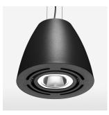
Suspended luminaire with LED, rated life of the LED L80/B10 > 50000 h, colour rendering index CRI > 80, chromaticity tolerance 2 SDCM (initial), reflector with circular light distribution pattern, reflector pure aluminium 99,99% in MIRO-Silver®, swivel angle +/-25°, luminaire housing sheet steel, powder-coated, black
