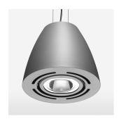
Suspended luminaire with LED, rated life of the LED L80/B10 > 50000 h, colour rendering index CRI > 90, chromaticity tolerance 2 SDCM (initial), reflector with oval light distribution pattern, reflector pure aluminium 99,99% in MIRO-Silver®, swivel angle +/-25°, luminaire housing sheet steel, powder-coated, silver
