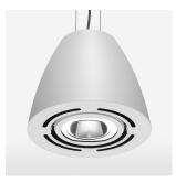
Suspended luminaire with LED, rated life of the LED L80/B10 > 50000 h, colour rendering index CRI > 80, chromaticity tolerance 2 SDCM (initial), reflector with circular light distribution pattern, reflector pure aluminium 99,99% in MIRO-Silver®, swivel angle +/-25°, luminaire housing sheet steel, powder-coated, white
