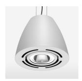
Suspended luminaire with LED, rated life of the LED L80/B10 > 50000 h, colour rendering index CRI > 80, chromaticity tolerance 2 SDCM (initial), reflector with circular light distribution pattern, reflector pure aluminium 99,99% in MIRO-Silver®, swivel angle +/-25°, luminaire housing sheet steel, powder-coated, white
