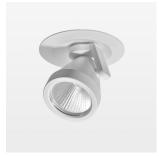
Semi-recessed luminaire with LED, rated life of the LED L80/B10 50000 h (tambient 25°C), colour rendering index CRI > 96, chromaticity tolerance 2 SDCM (initial), reflector with circular light distribution pattern, reflector pure aluminium 99,99% in MIRO-Silver®, segmented and faceted, 3D lens silicon to reduce the proportion of scattered light, die-cast aluminium, powder-coated, rotation angle 400°, swivel angle +/- 85°, white, separate driver unit
