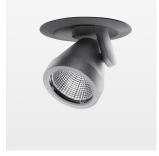
Semi-recessed luminaire with LED, rated life of the LED L80/B10 50000 h (tambient 25°C), colour rendering index CRI > 96, chromaticity tolerance 2 SDCM (initial), reflector with circular light distribution pattern, reflector pure aluminium 99,99% in MIRO-Silver®, segmented and faceted, 3D lens silicon to reduce the proportion of scattered light, die-cast aluminium, powder-coated, rotation angle 400°, swivel angle +/- 85°, silver, separate driver unit
