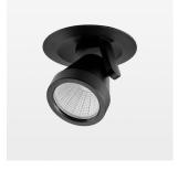
Semi-recessed luminaire with LED, rated life of the LED L80/B10 50000 h (tambient 25°C), colour rendering index CRI > 96, chromaticity tolerance 2 SDCM (initial), reflector with circular light distribution pattern, reflector pure aluminium 99,99% in MIRO-Silver®, segmented and faceted, 3D lens silicon to reduce the proportion of scattered light, die-cast aluminium, powder-coated, rotation angle 400°, swivel angle +/- 85°, black, separate driver unit
