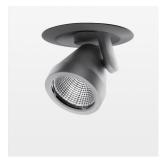
Semi-recessed luminaire with LED, rated life of the LED L80/B10 50000 h (tambient 25°C), colour rendering index CRI > 95, chromaticity tolerance 2 SDCM (initial), rotation-symmetrical reflector with circular light distribution pattern, reflector pure aluminium 99,99% in MIRO-Silver®, segmented and faceted, 3D lens silicon to reduce the proportion of scattered light, die-cast aluminium, powder-coated, rotation angle 400°, swivel angle +/- 85°, silver, separate driver unit
