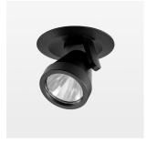
Semi-recessed luminaire with LED, rated life of the LED L80/B10 50000 h (tambient 25°C), colour rendering index CRI > 95, chromaticity tolerance 2 SDCM (initial), rotation-symmetrical reflector with circular light distribution pattern, reflector pure aluminium 99,99% in MIRO-Silver®, segmented and faceted, 3D lens silicon to reduce the proportion of scattered light, die-cast aluminium, powder-coated, rotation angle 400°, swivel angle +/- 85°, black, separate driver unit
