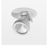
Semi-recessed luminaire with LED, rated life of the LED L80/B10 50000 h (tambient 25°C), colour rendering index CRI > 96, chromaticity tolerance 2 SDCM (initial), reflector with circular light distribution pattern, reflector pure aluminium 99,99% in MIRO-Silver®, segmented and faceted, 3D lens silicon to reduce the proportion of scattered light, die-cast aluminium, powder-coated, rotation angle 400°, swivel angle +/- 85°, white, potentiometer to adjust the brightness, separate driver unit
