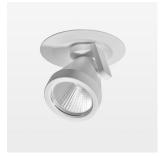
Semi-recessed luminaire with LED, rated life of the LED L80/B10 50000 h (tambient 25°C), colour rendering index CRI > 80, chromaticity tolerance 2 SDCM (initial), reflector with circular light distribution pattern, reflector pure aluminium 99,99% in MIRO-Silver®, segmented and faceted, 3D lens silicon to reduce the proportion of scattered light, die-cast aluminium, powder-coated, rotation angle 400°, swivel angle +/- 85°, white, potentiometer to adjust the brightness, separate driver unit
