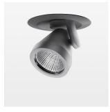
Semi-recessed luminaire with LED, rated life of the LED L80/B10 50000 h (tambient 25°C), colour rendering index CRI > 96, chromaticity tolerance 2 SDCM (initial), reflector with circular light distribution pattern, reflector pure aluminium 99,99% in MIRO-Silver®, segmented and faceted, 3D lens silicon to reduce the proportion of scattered light, die-cast aluminium, powder-coated, rotation angle 400°, swivel angle +/- 85°, silver, potentiometer to adjust the brightness, separate driver unit
