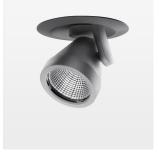
Semi-recessed luminaire with LED, rated life of the LED L80/B10 50000 h (tambient 25°C), colour rendering index CRI > 80, chromaticity tolerance 2 SDCM (initial), reflector with circular light distribution pattern, reflector pure aluminium 99,99% in MIRO-Silver®, segmented and faceted, 3D lens silicon to reduce the proportion of scattered light, die-cast aluminium, powder-coated, rotation angle 400°, swivel angle +/- 85°, silver, potentiometer to adjust the brightness, separate driver unit
