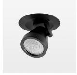
Semi-recessed luminaire with LED, rated life of the LED L80/B10 50000 h (tambient 25°C), colour rendering index CRI > 90, chromaticity tolerance 2 SDCM (initial), reflector with circular light distribution pattern, reflector pure aluminium 99,99% in MIRO-Silver®, segmented and faceted, 3D lens silicon to reduce the proportion of scattered light, die-cast aluminium, powder-coated, rotation angle 400°, swivel angle +/- 85°, black, potentiometer to adjust the brightness, separate driver unit
