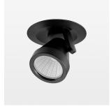
Semi-recessed luminaire with LED, rated life of the LED L80/B10 50000 h (tambient 25°C), colour rendering index CRI > 96, chromaticity tolerance 2 SDCM (initial), reflector with circular light distribution pattern, reflector pure aluminium 99,99% in MIRO-Silver®, segmented and faceted, 3D lens silicon to reduce the proportion of scattered light, die-cast aluminium, powder-coated, rotation angle 400°, swivel angle +/- 85°, black, potentiometer to adjust the brightness, separate driver unit
