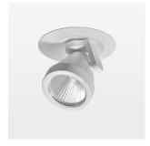
Semi-recessed luminaire with LED, rated life of the LED L80/B10 50000 h (tambient 25°C), colour rendering index CRI > 96, chromaticity tolerance 2 SDCM (initial), reflector with circular light distribution pattern, reflector pure aluminium 99,99% in MIRO-Silver®, segmented and faceted, 3D lens silicon to reduce the proportion of scattered light, die-cast aluminium, powder-coated, rotation angle 400°, swivel angle +/- 85°, white, separate driver unit
