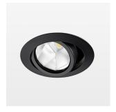
Recessed luminaire with LED, rated life of the LED L80/B10 50000 h (tambient 25°C), colour rendering index CRI > 96, chromaticity tolerance 2 SDCM (initial), reflector with oval light distribution pattern, reflector pure aluminium 99,99% in MIRO-Silver®, segmented, die-cast aluminium, powder-coated, rotation angle, swivel angle +/- 25°, black,
