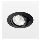
Recessed luminaire with LED, rated life of the LED L80/B10 50000 h (tambient 25°C), colour rendering index CRI > 90, chromaticity tolerance 2 SDCM (initial), reflector with oval light distribution pattern, reflector pure aluminium 99,99% in MIRO-Silver®, segmented, die-cast aluminium, powdercoated, rotation angle, swivel angle +/- 25°, black,
