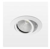
Recessed luminaire with LED, rated life of the LED L80/B10 50000 h (tambient 25°C), colour rendering index CRI > 96, chromaticity tolerance 2 SDCM (initial), reflector with circular light distribution pattern, reflector pure aluminium 99,99% in MIRO-Silver®, segmented and faceted, die-cast aluminium, powder-coated, rotation angle, swivel angle +/- 25°, white,
